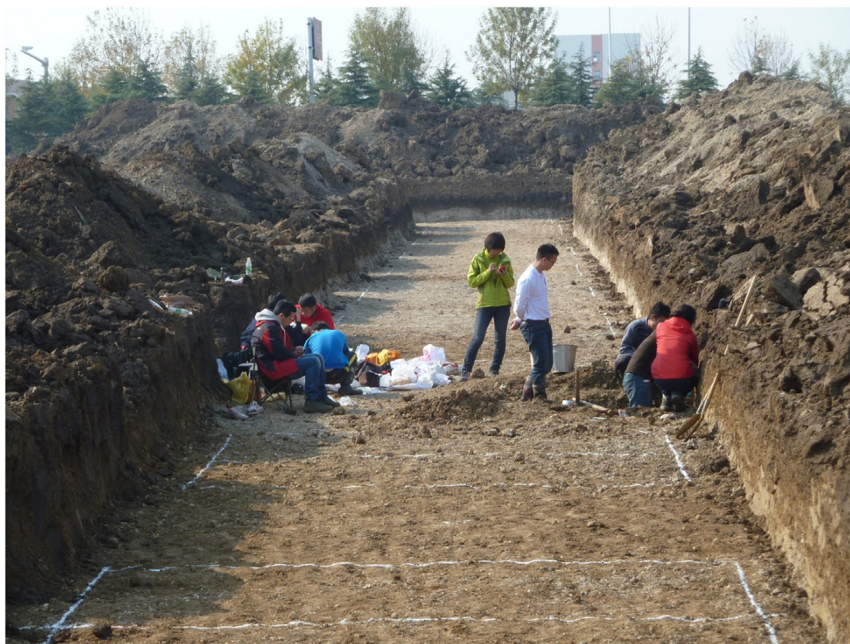
Fig. 1 Soil profile description and sampling at an excavation for building foundation, HeDong neighborhood, LinYi City, Shandong Province, China (34.996N 118.48E). Note the good view of the horizontal and vertical spatial variability of the horizons.
