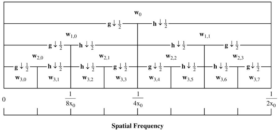
**Figure 2** The discrete wavelet packet transform (DWPT) as an even partition of the spatial frequency range by successive passes of scaling function and wavelet function filters.
