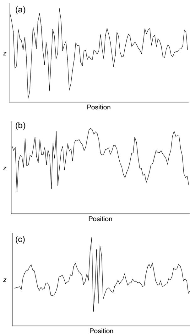
**Figure 1** Three hypothetical transects on which the data appear inconsistent with an assumption of underlying stationarity: (a) there is a change in variance (but the autocorrelation remains unchanged); (b) there is a change in the autocorrelation function (but not in the variance); and (c) a realization of a stationary process is interrupted by a distinctive local pattern of variation.
