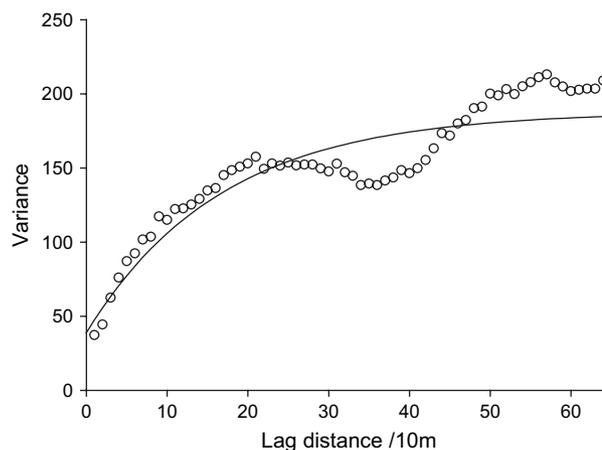
**Figure 5** Experimental variogram (symbols) and fitted exponential model (line). The model is given in Equation (13).
