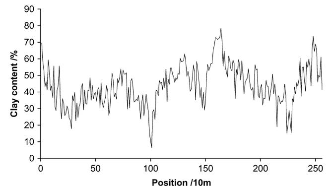
**Figure 8** One realization, at the sample sites on the Sandford transect, of a stationary random variable with the same variogram as the data on topsoil clay content.
