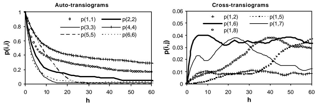
**Fig. 1.** Some transiograms estimated from a soil type map in the west-east direction.  $p(i,j)$  in legends means a transiogram from class  $i$  to  $j$ . Scales along the  $h$  axis are numbers of grid units in the direction.
